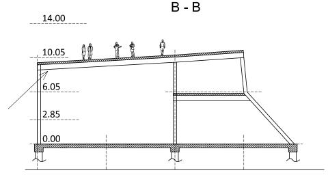
Long span composite steel-reinforced concrete structure to follow roof and facade shape and to support pedestrian loads
